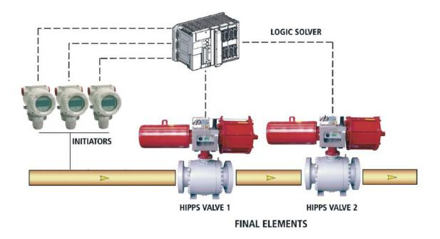
The above schematic is a typical HIPPS architecture. The solver will decide based on 2-out-of-3 (2003) voting whether or not to activate the final element. The final elements consist here of two block valves that stop flow to the downstream facilities to prevent them from exceeding a maximum pressure. The components in the loop can vary according to customer specification and requirement.
